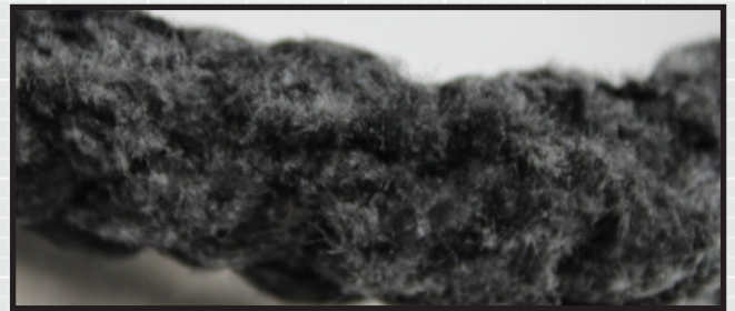
Picture 12: Severe wear of extraction loop.
