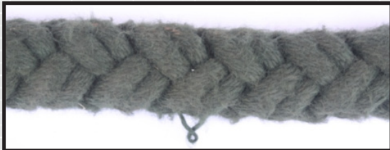
Picture 2: Hooked yarn under 25mm
