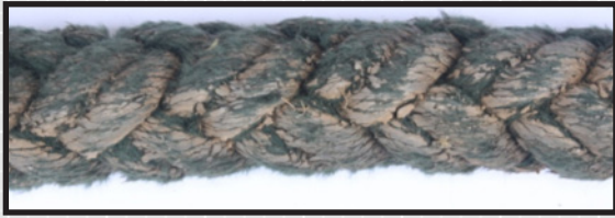
Picture 1: Muddy rope should be cleaned
