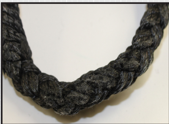
Picture 11: Normal surface abrasion on extraction loop.
